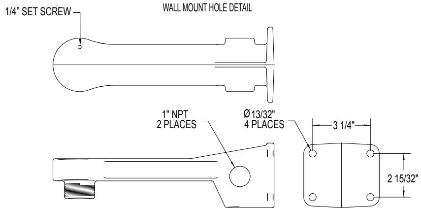
Securely tighten set screws when desired fixture orientation is achieved and the conduit connection is tight.
