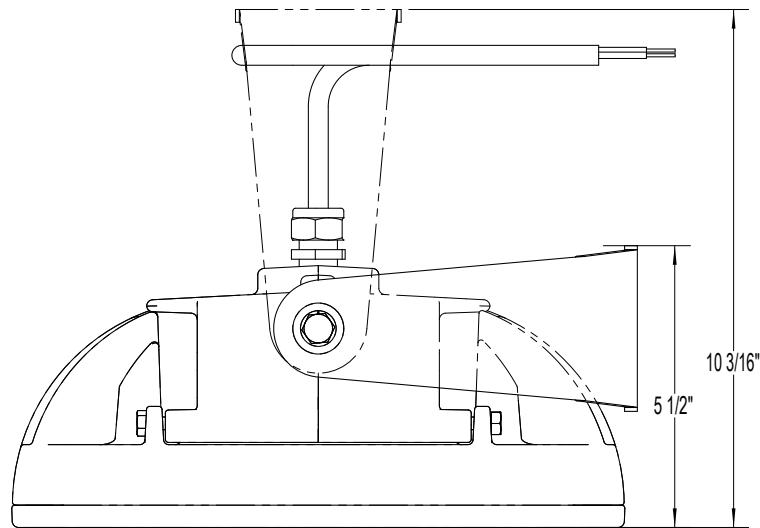
**NOTE:** It is not necessary to remove the yoke mount to install the fixture. If removal of the yoke mount is required, remove the lock nut from each side of the yoke and flex the yoke bracket off of the Set Screw/Studs.
