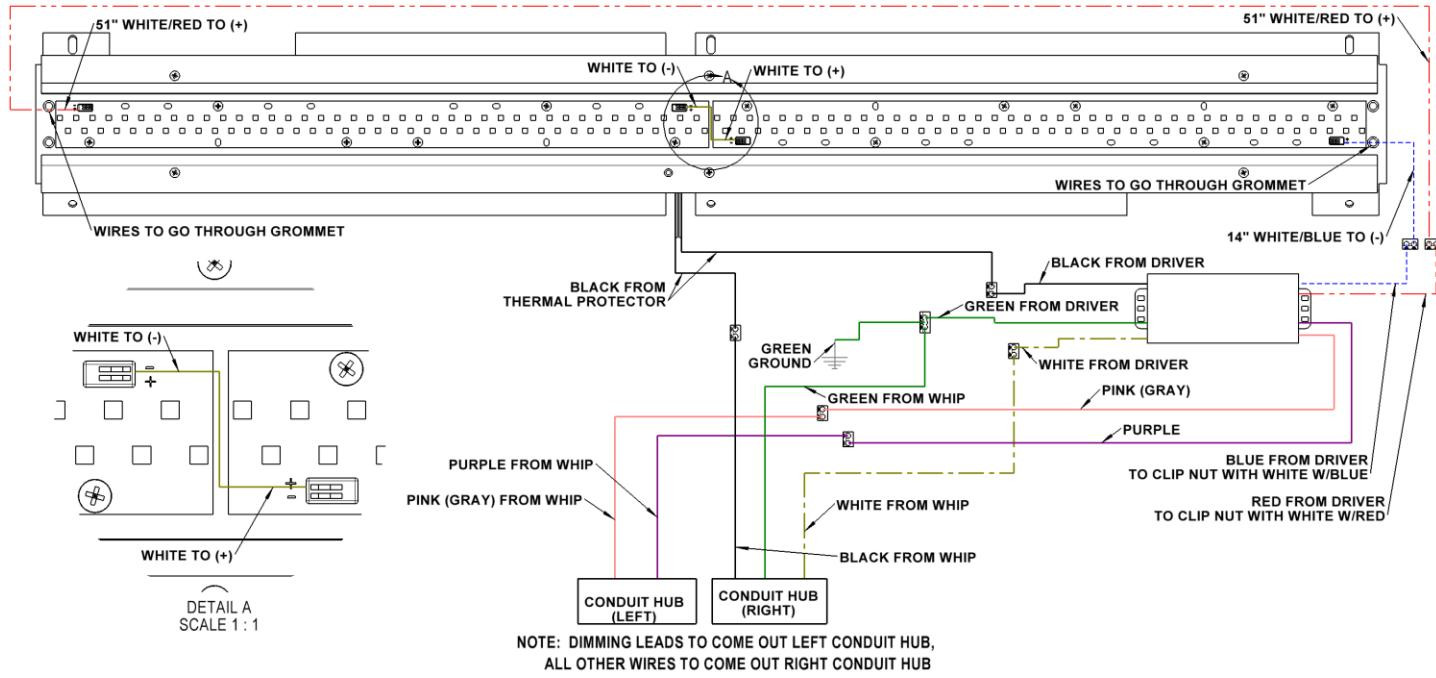
\*\*Note - Basic Schematic, including dimming leads. Surge protection device and EM option not shown here.\*\*
