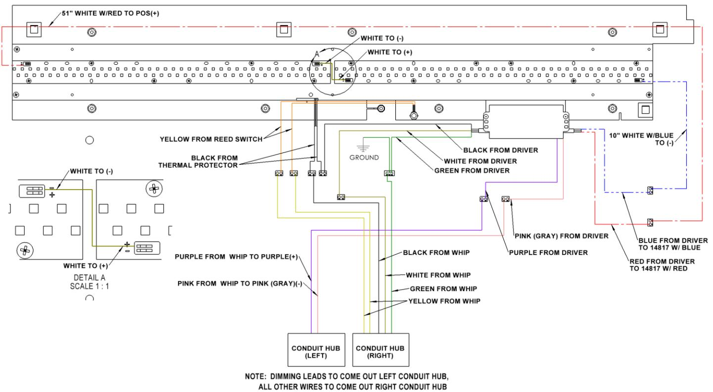
\*\*Note - Basic Schematic, including as dimming leads and reed switch, surge protection device and EM option not shown here.\*\*
