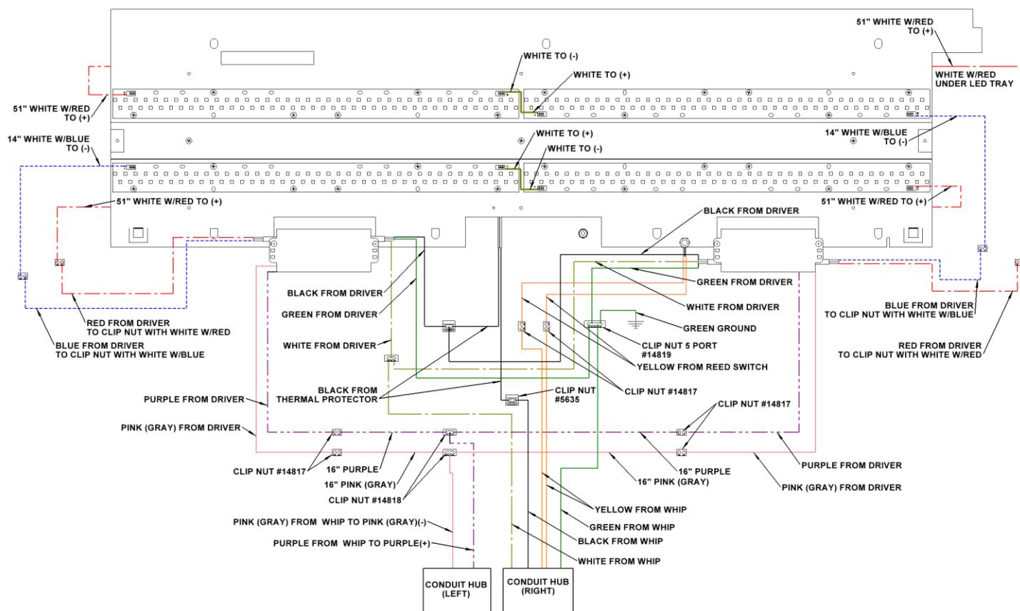
\*\*Note - Basic Schematic, including reed switch. Dimming leads, surge protection device and EM option not shown here.\*\*
